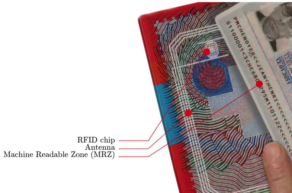
Figure 12.14. E-passport Main Components (source: www.passeportsuisse.ch )
