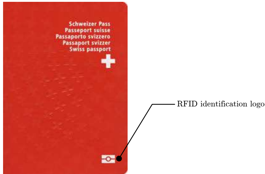
Figure 12.13. How to Distinguish an E-passport? (source: www.passeportsuisse.ch )
